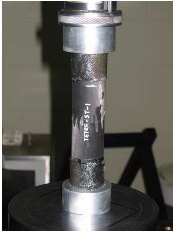
Figure 13. Graphite/Epoxy Seat Tube After Impact and Compression Testing
