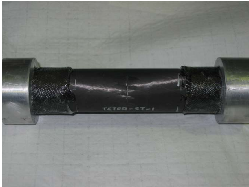
Figure 12. Graphite/Epoxy Seat Tube After Impact
