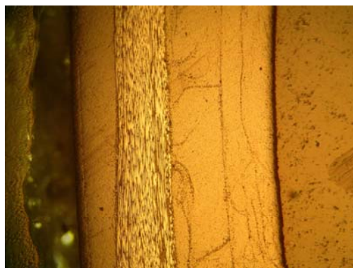
Figure 3. Cross-Sectional View of Graphite/Epoxy Seat Tube
