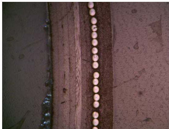
Figure 5. Cross-Sectional View of Hy-Bor Seat Tube
