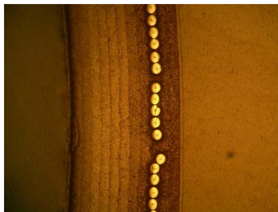
Figure 6. Cross-Sectional View of Hy-Bor Down Tube
